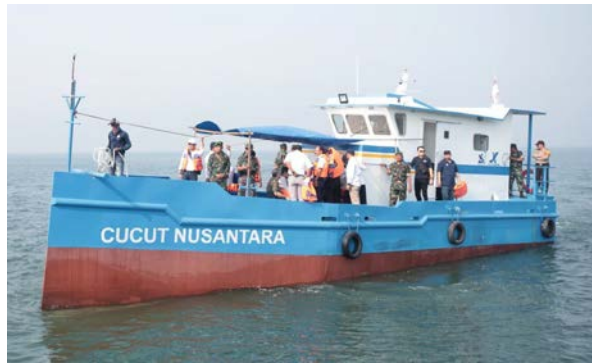
Fig. 1 The "Cucut Nusantara" Flat-sided Hull boat developed by the University Indonesia and Juragan Kapal Indonesia Corp [8]
