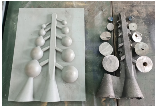
Fig. 6. Casting model and section
