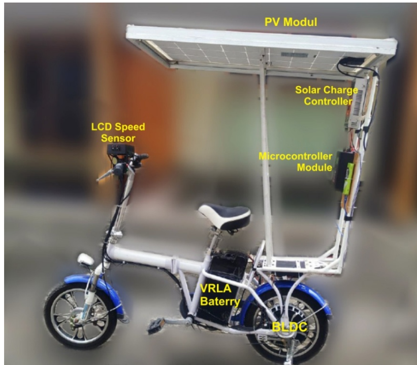
Fig. 2. The prototype of hybrid solar e-bike
