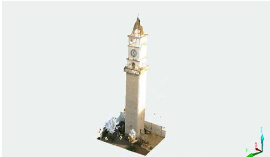
Fig. 4. TLS Point Cloud generated in Faro Scene
