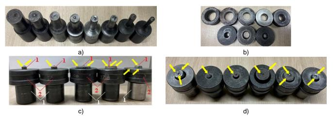
Fig. 2. Worn busbar punching tools: a – busbar punching tools; b – punches; c, d – assembled busbar punching tools; 1 – busbar punching tool; 2 – punch; - wear and chips
