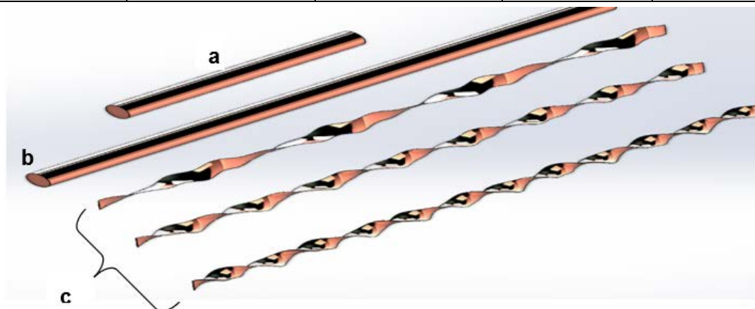
Fig.1. (a) entrance, (b) test tube and (c) modified twisted tapes
