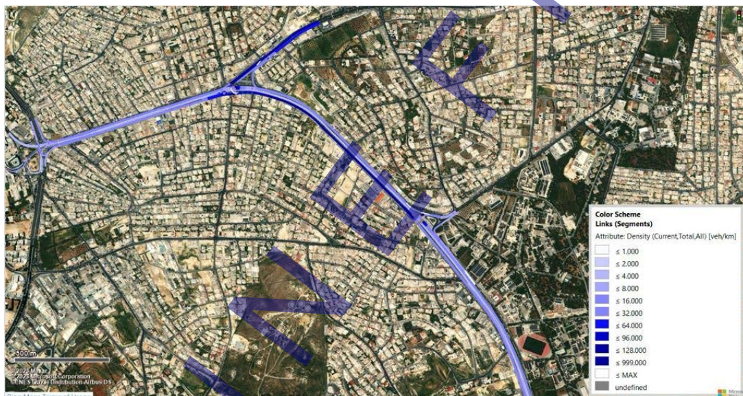
Fig. 16. The density in (vehicle/km) of the whole network for the proposed situation (scenario) adopted from PTV Vissim
