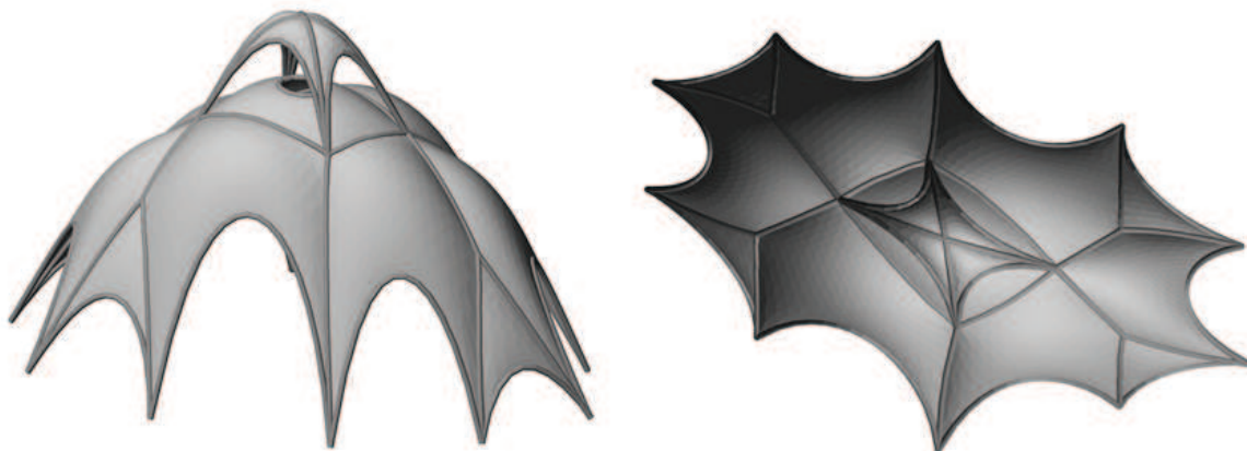
Figure 5: Two-storey compression structure computed using TM-FDM: general (left) and plan (right) views
