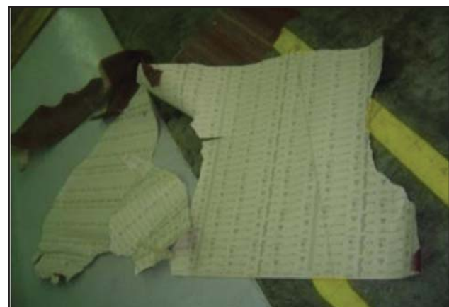
Figure 8: Examples of broken sanding papers
