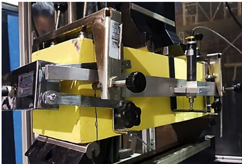
Fig. 5. Beam clamping device, for LDT transducers and VPU transducers. Source: Authors.
