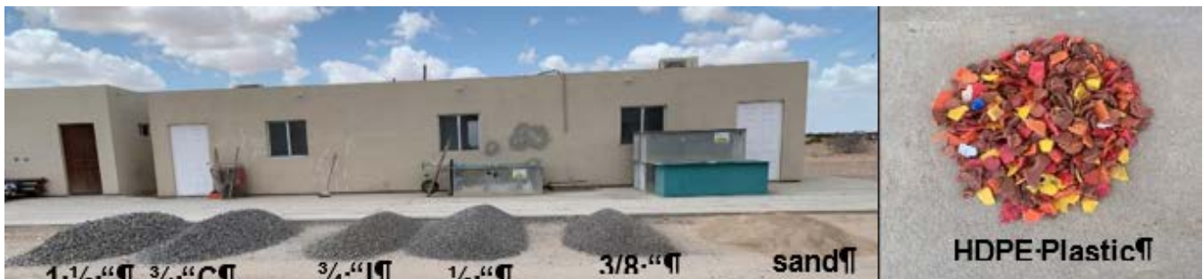
Fig. 2. Granulometric distribution of HDPE plastic. Own elaboration
