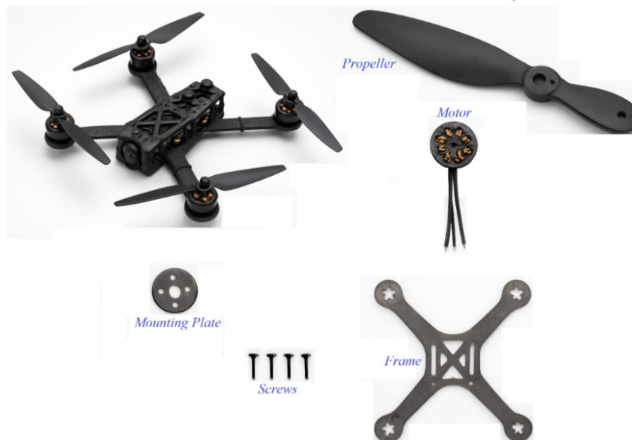
Fig. 4. Structural components of a drone made from carbon composite materials
