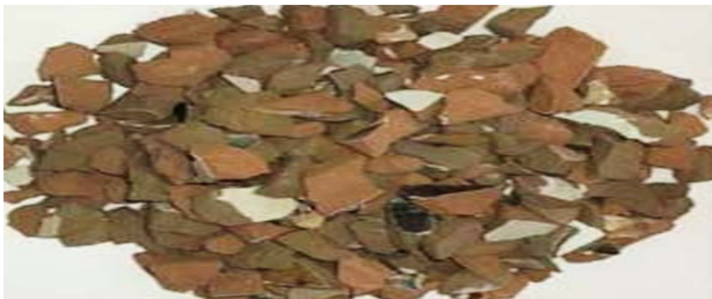
Fig. 1. Ceramic recycled coarse aggregates (RCA)
