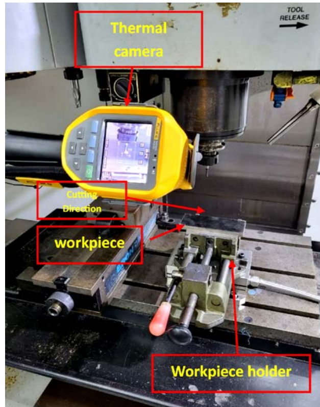
Fig. 2. The CNC milling cutting direction
