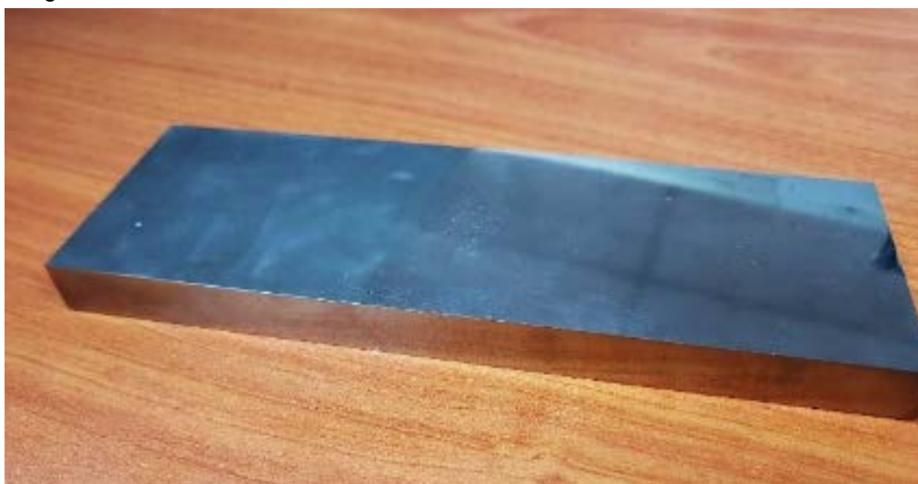
Fig. 1. The SLM-produced Ti-6Al-4V specimens used in this study
