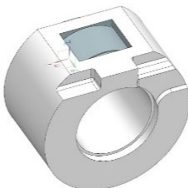
Fig. 9. Calculated part: support bushing with a plate (expanding element)
