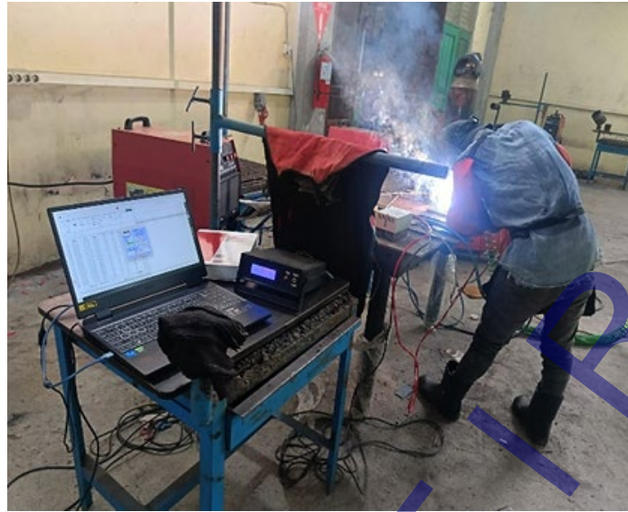
Fig. 3. Shielded metal arc welding (SMAW) process
