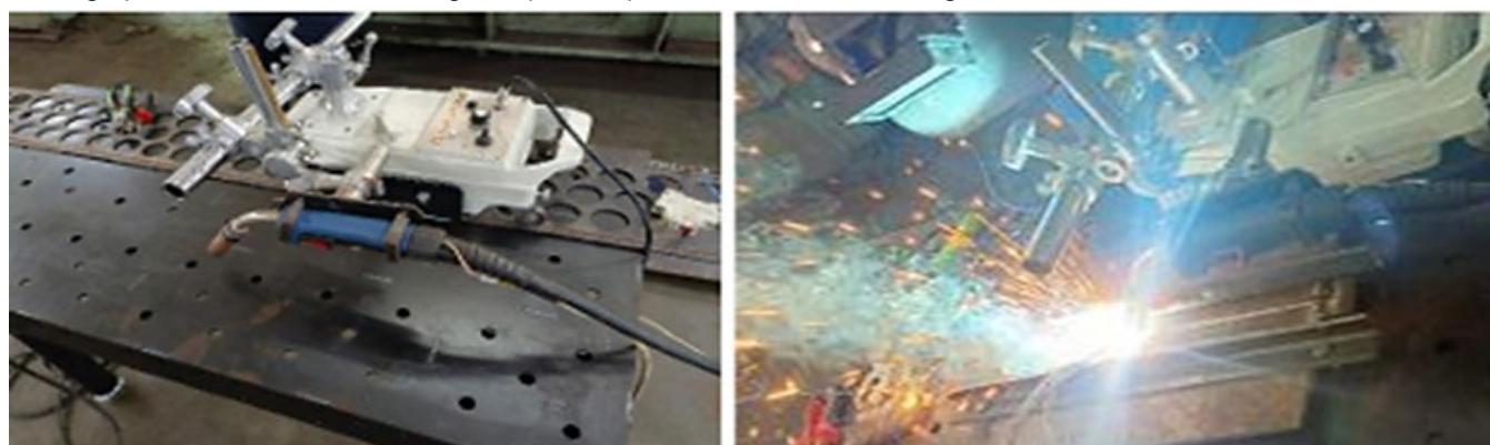
Fig. 2. Robotic GMAW welding: (a) welding setup and (b) welding operation
