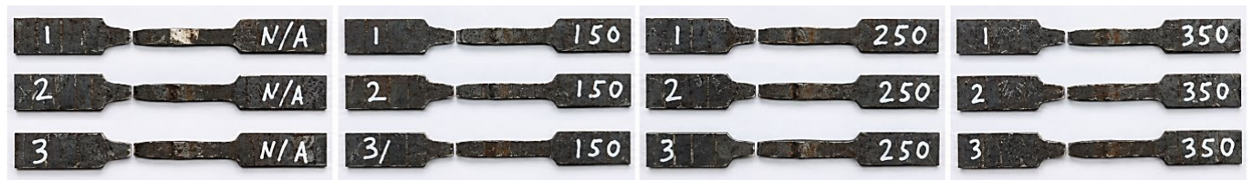
Fig. 8. Post-fracture tensile specimens under different preheating conditions
