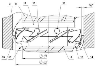
Figure 5: Scheme of the vane wheel arrangement
