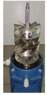
Figure 7: Photograph of the experimental rotor model
