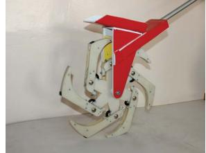
Figure 11: Picture of universal walking wheel model
