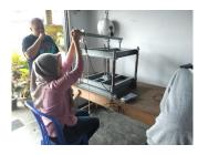
Figure 1: Pressing machine to mold the cassava dough
