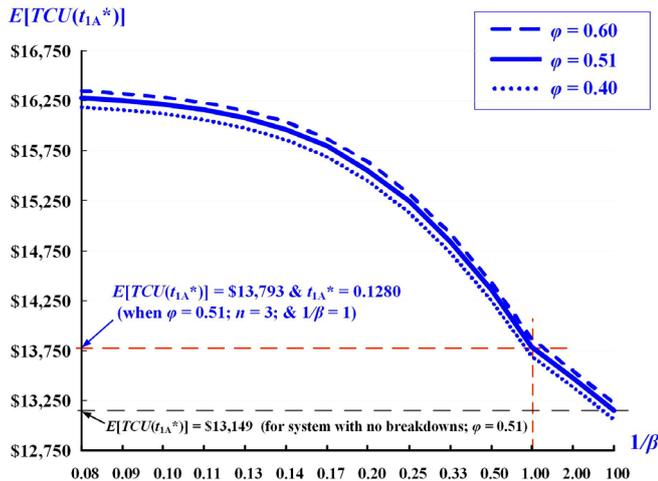
Figure 7: The influence of differences in  $1/\beta$  with different  $\phi$  on  $E[TCU(t_{1A}^*)]$
