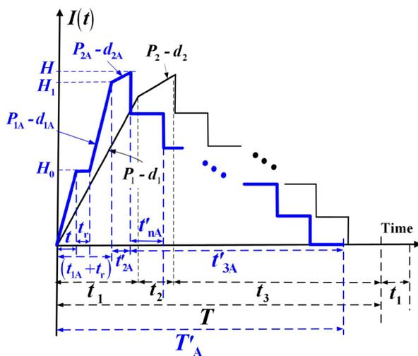
Figure 1: Level of perfect stocks in the proposed coordinated vendor-buyer system with an expedited rate, unreliable machine, scrap, and rework (in blue) as compared to that of the same system without expedited rate, nor machine failure (in black)
