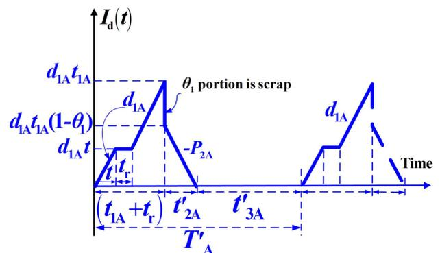
Figure 3: Level of nonconforming stocks in situation one
