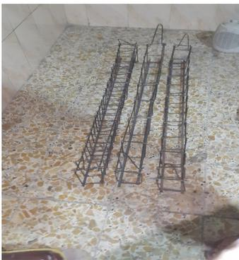
Figure 4: Steel reinforcement
