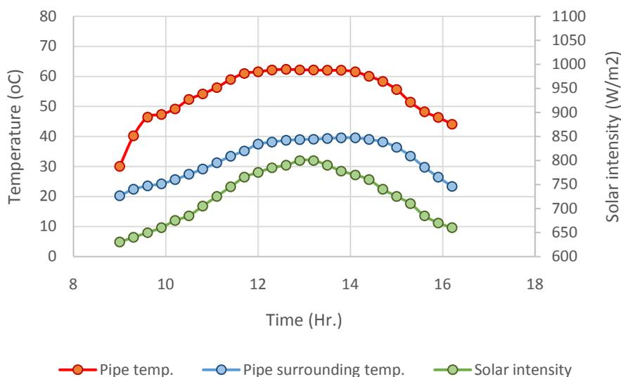
Figure 4. Heat pipe system temperatures and incoming solar intensity with no cover case
