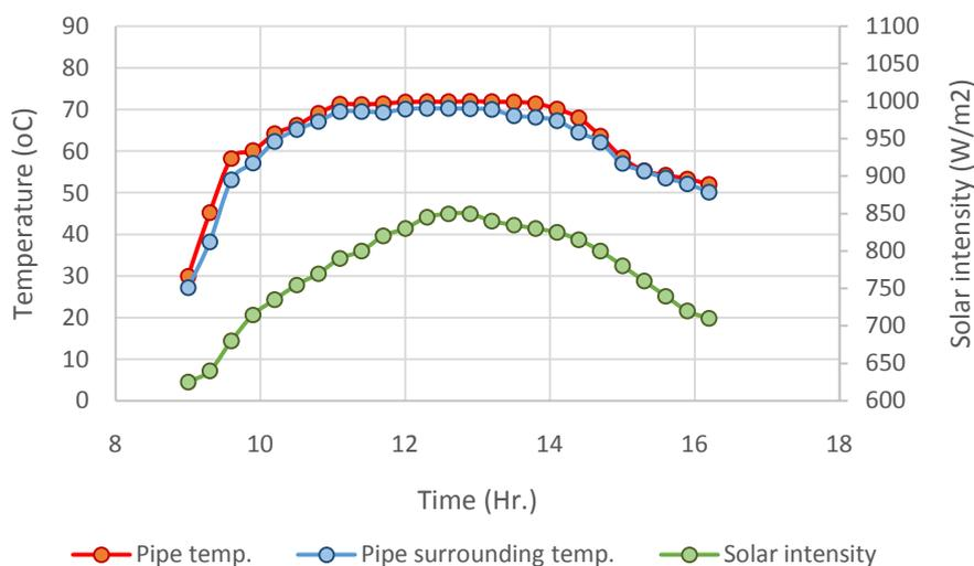
Figure 5. Heat pipe system temperatures and incoming solar intensity with the double cover case.
