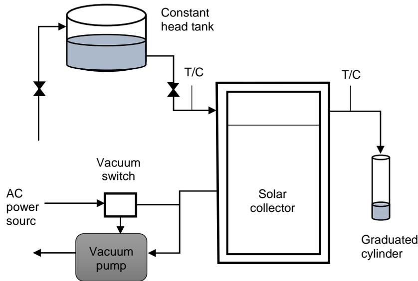
Figure 3. Schematic diagram of the experimental system
