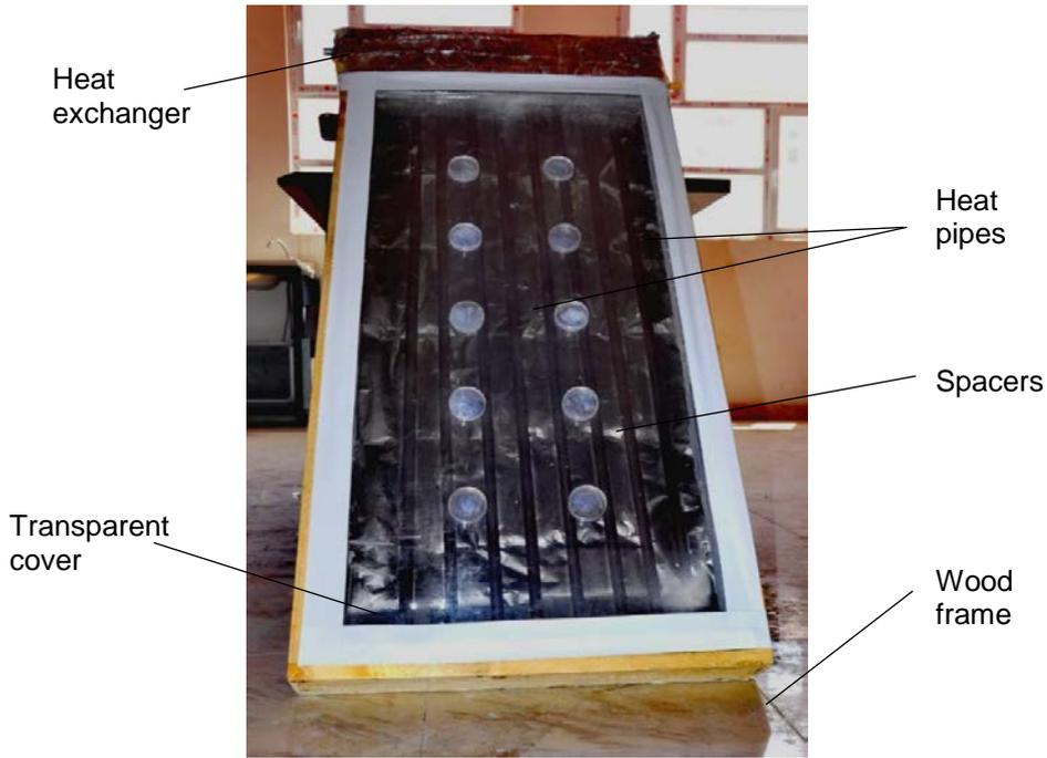
Figure 1. The final layout of the solar collector.
