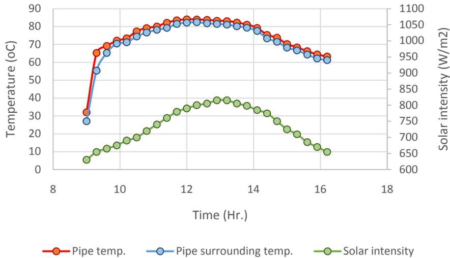
Figure 6. Heat pipe system temperatures and incoming solar intensity with the vacuumed double cover case.
