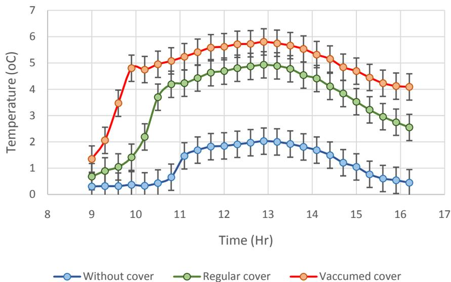
Figure 7. Water temperature difference variation with time for the three solar panel cases
