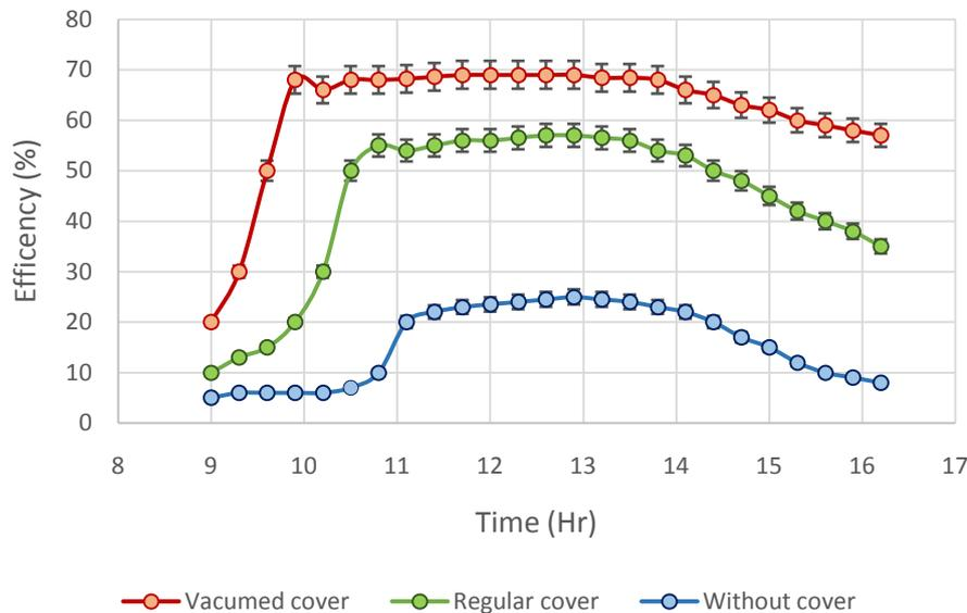
Figure 8. Variation of solar collector efficiency with time for the three cases of the study
