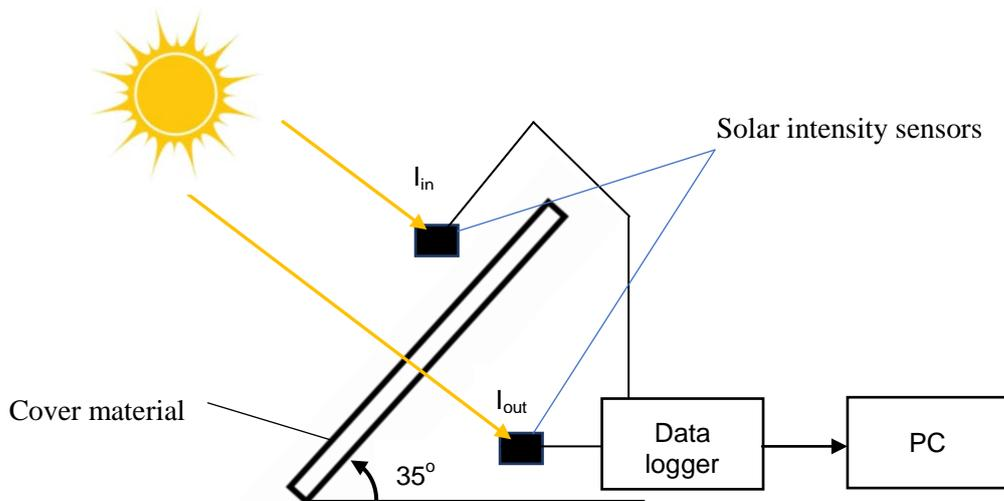
Figure 2. Schematic diagram for the layout used in the tests to calculate solar loss
