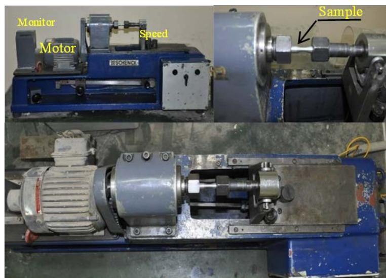
Fig.4. Equipment of the rotating bending fatigue testing machine (a Schenck product) that has the fatigue sample test attached to it. (a) side view of the rotating bending fatigue testing machine; (b) top view of the rotating bending fatigue testing machine
