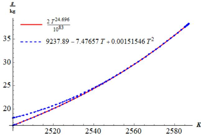
Fig. 2. NO<sub>x</sub> levels. The red line shows an exponential growth of NO<sub>x</sub> as a function of temperature, while the blue dashed line shows an approximately quadratic behavior
