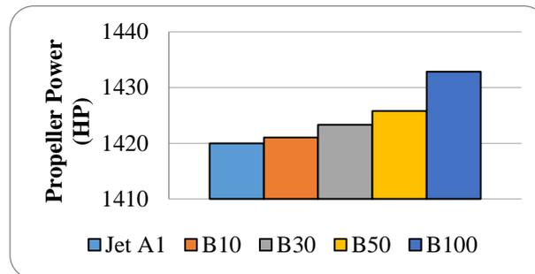
Fig. 5. Comparison of propeller power
