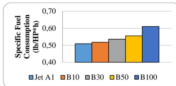
Fig. 6. Comparison of Specific Fuel Consumption
