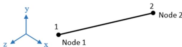
Fig. 2. 2-noded 3D linear truss element
