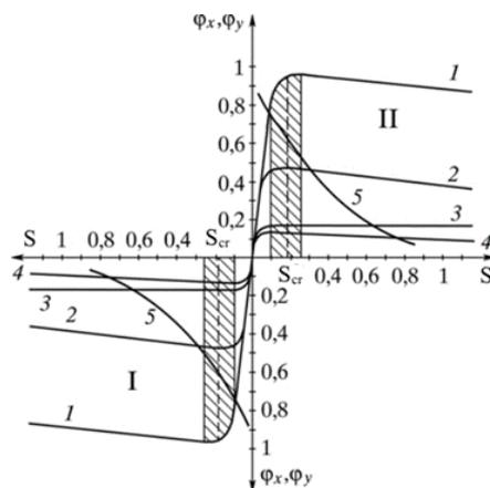
Fig. 1. Diagrams of the relationship between the traction coefficient and wheel slip. I, II – traction and braking modes, respectively, 1 – dry asphalt, 2 – wet concrete, 3 – wet paving stone, 4 – rolled snow, 5 – cross direction for dry asphalt.
