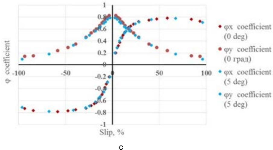
Fig. 4. Experimental diagrams of the variation of adhesion coefficients from sliding. a – R<sub>z</sub> 4000H, b – R<sub>z</sub> 6000H, c – R<sub>z</sub> 8000H
