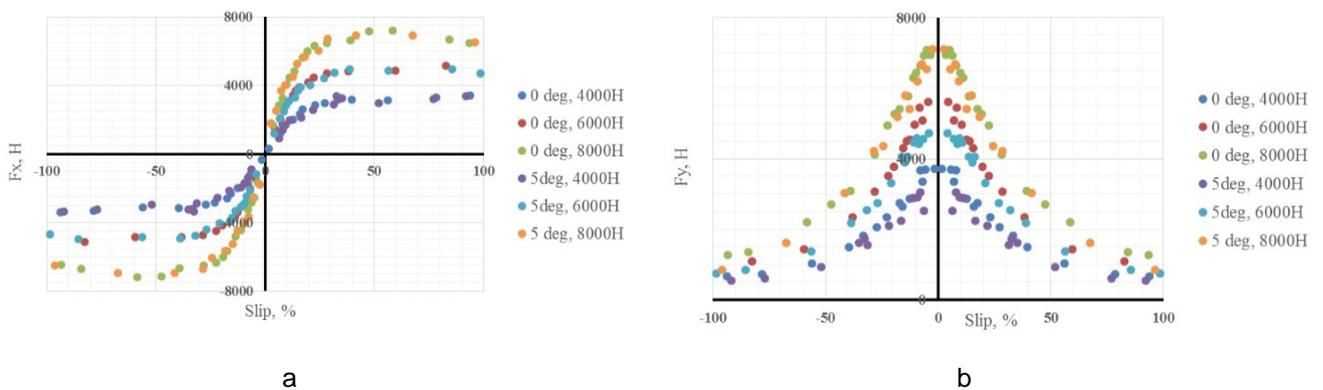
Fig. 5. Experimental graphs of changes in longitudinal (Fx) and lateral (Fy) forces from sliding at different vertical loads and slip angles
