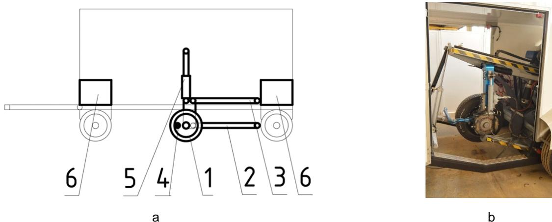
Fig. 3. Tire test bench used by NNSTU. a - Schematic diagram of a trail lab for the study of the dynamic characteristics of tires, b – Prototype of a trail lab. 1 – the studied tire; 2 – lower arm; 3 – upper arm; 4 – electrohydraulic drive of the slip angle; 5 – vertical force electrohydraulic drive on the wheel; 6 – ballast
