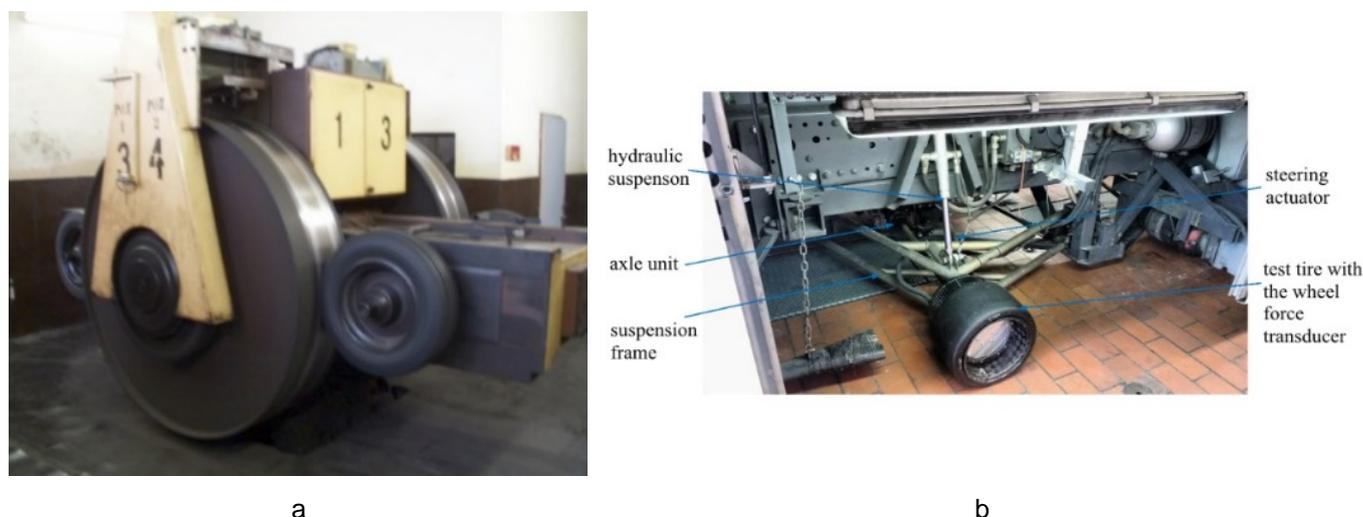
Fig. 2. Tire test benches. a – stationary [17], b – road [19]
