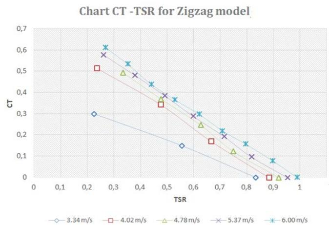
Fig. 8.  $C_T$  – TSR for Model I
