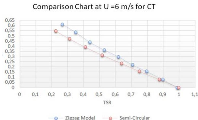
Fig. 12. Comparison  $C_T$  - TSR for Model I with Model II at U= 6 m/s
