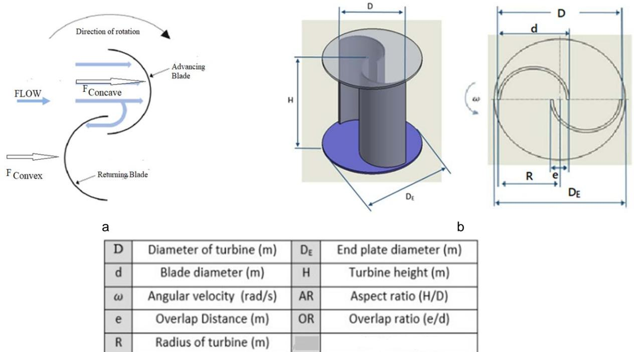
Fig. 1. The simple construction of Savonius (a) Working principle (b) Geometry
