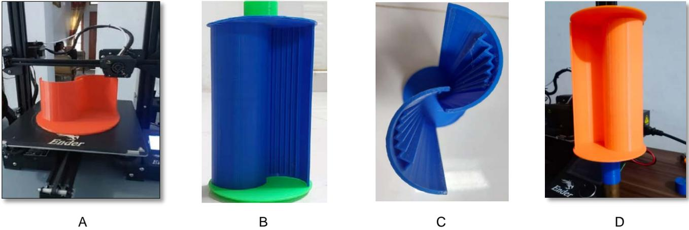
Fig. 3. (a) The process of printing models (b) (Front view of model I (c) Top View of Model I (d) Model II
