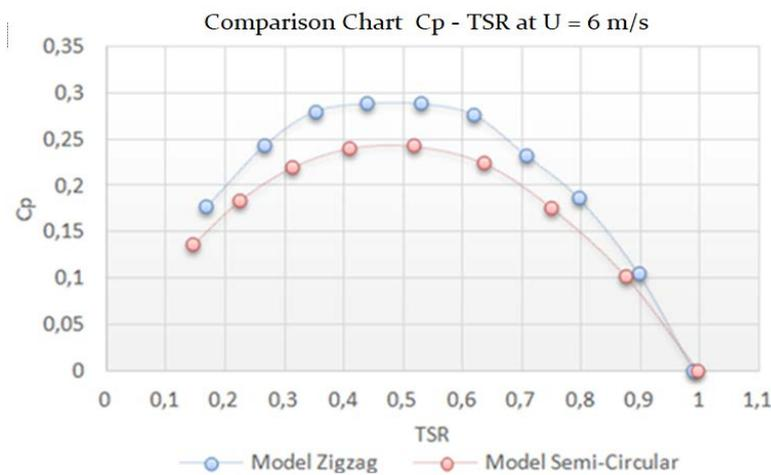
Fig. 11. Comparison Cp-TSR for Model I and Model II at U=6 m/s
