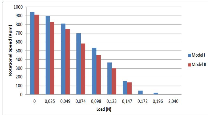
Fig. 6. Char Load – Rotational Speed
