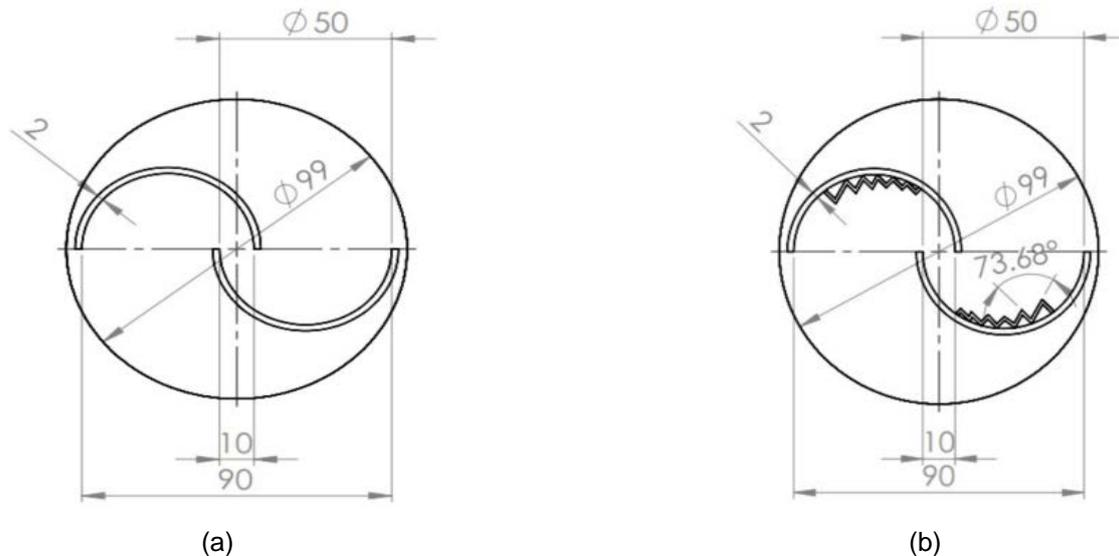
Fig. 2. Dimension of model savonius a) Semi-circular Savonius b) Savonius with Using Tiered-Height Zigzag
