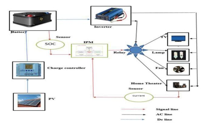
Figure 5: Schematic diagram of Intelligent Power Management(IPM)
