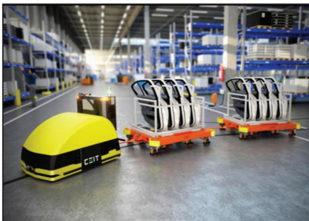
Figure 5: AGV system – towing version
