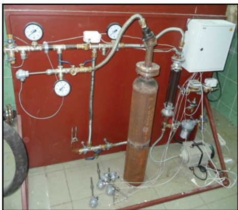
Figure 2: The experimental equipment for the study of the functioning of the catalytic combustion system
