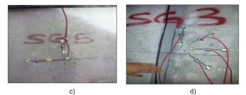
Figure 6: Installation of Vibrating Wire Strain Gauges (VWSGs) at mid-span area; (a) Data logging equipment set up at desk; (b) Bottom top slab gauge arrangement at SG7; (c) Bottom slab gauge arrangement at SG5; and (d) Web gauge arrangement at SG3
