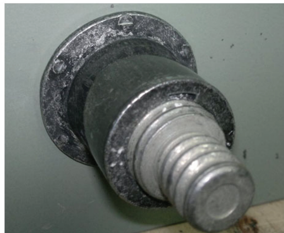
Figure 5: Installation indicators on collar flange before and after installation
