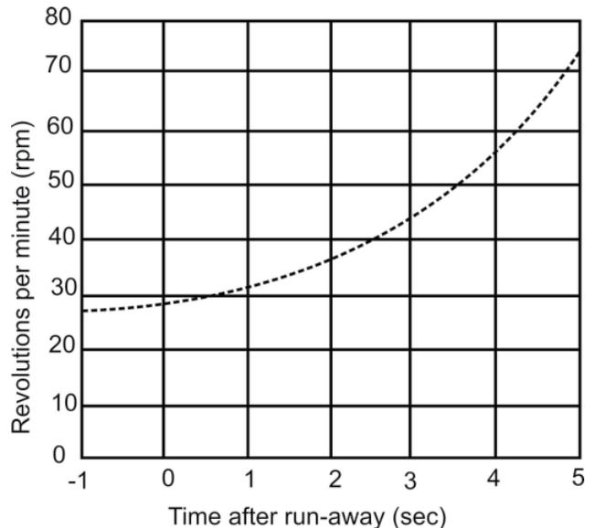
Fig. 6. Revolution per minute in run-away state
