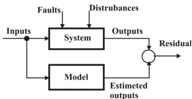
Fig. 2. Fault estimation based in residual
