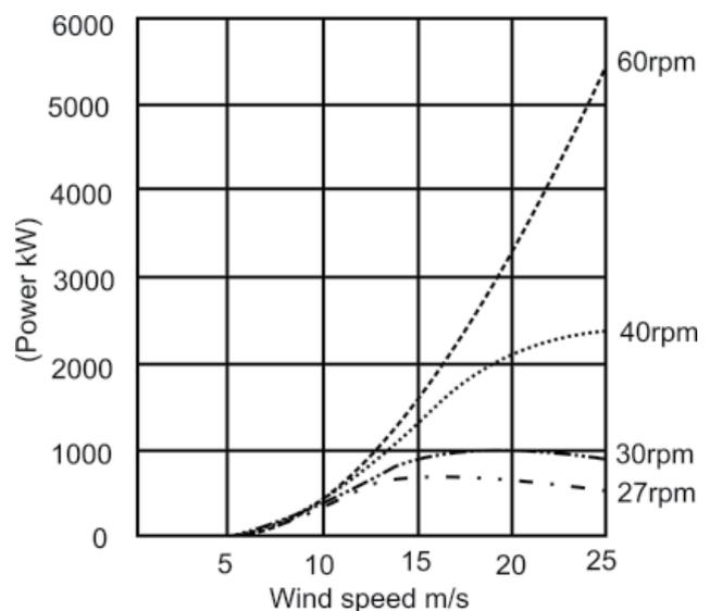
Fig. 5. Power curves depends of wind speed and wind turbine angular velocity
