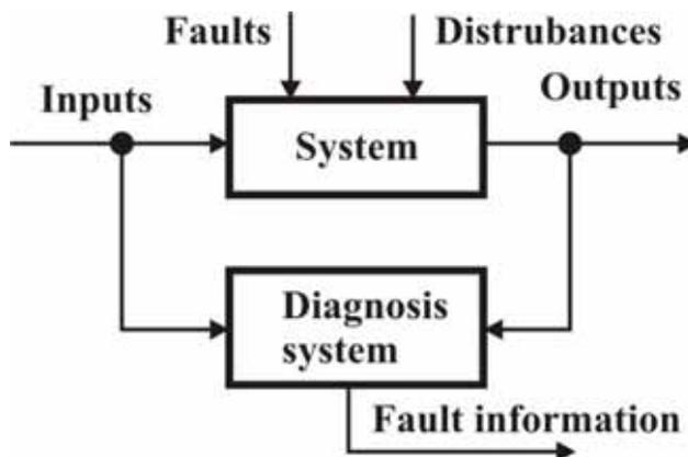
Fig. 1. Principle of model based fault detection
