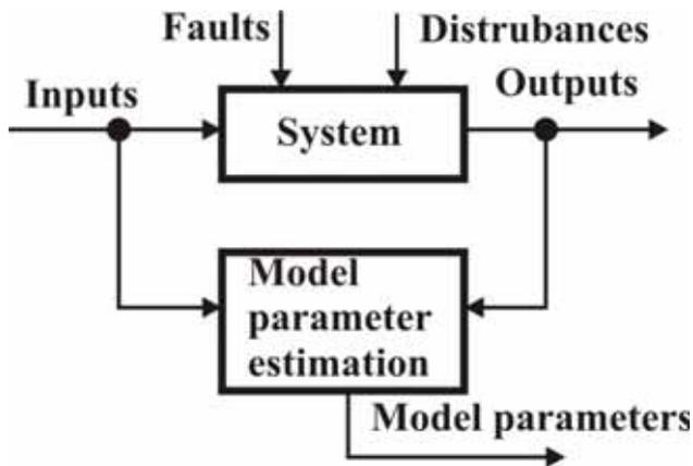
Fig. 3. Fault estimation based on model parameters
